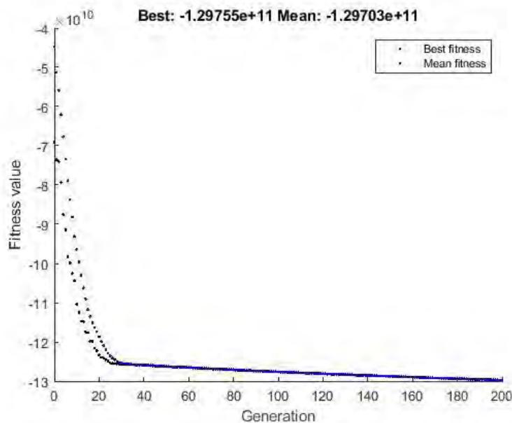
The convergence chart of the genetic algorithm in Figure1 illustrates the improvement trend of the objective function over 200 generations. The chart displays the number of generations on the horizontal axis and the objective function value on the vertical axis, with two primary curves: one representing the best fitness value and the other the mean fitness of the population. The vertical axis scale ranges from  $-13 \times 10^{10}$  to  $-4 \times 10^{10}$ , indicating a minimization problem.
