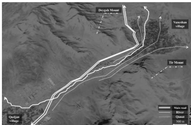
Fig. 3. Aerial photo path of three Qanat of Vaneshan, whose origins are in Qud-Jan village in Khansar province
