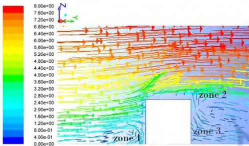
Fig. 5: graduating air velocity around a simple volume type A on the ground.
