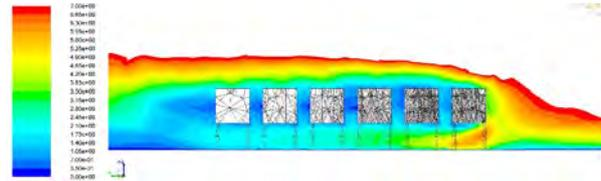
Fig. 12: Wind velocity contours around buildings in an urban length E with six rows.
