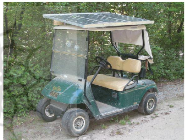
Fig.8: Golf car with batteries charged by solar panels in Earthaven
