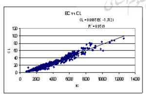
Figure 4: EC via Chloride ion
