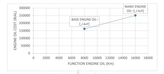
Figure 3. Comparing cost and performance of Nano engine oil
